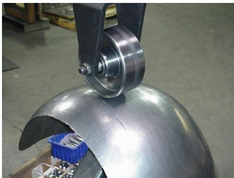
Figure 16: Picture of an English wheel with a doubly curved workpiece.
