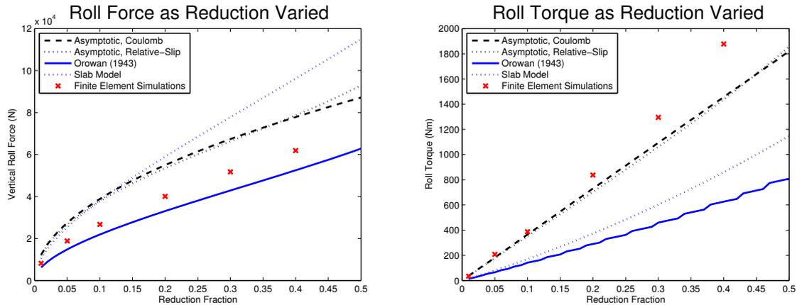
Figure 2: Results from a poster presentation at SNSCC-2014 showing a comparison of analytical models with finite element simulation results. Vertical roll force (left) and roll torque (right) as the workpiece reduction is varied.
