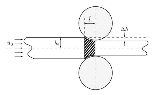
Figure 1: A not to scale diagram of a symmetric roller set-up, highlighting the plastic region to be solved (shaded) and other key parameters.
