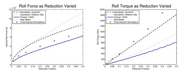
Figure 2: Results from a poster presentation at SNSCC-2014 showing a comparison of analytical models with finite element simulation results. Vertical roll force (left) and roll torque (right) as the workpiece reduction is varied.
